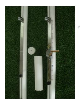
Tightening/tensioning of the net by means of rack jack.
