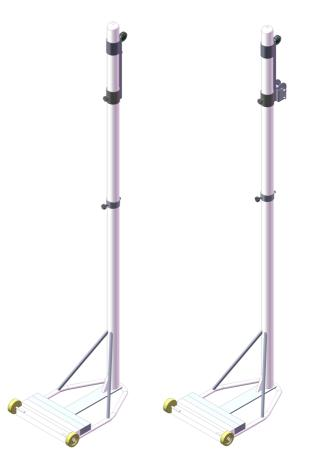
At the bottom, the posts are welded to the base. The base is composed of a tubular profile attached to the rear where the counterweights are welded, which secure the posts fixation. These counterweights are fitted with wheels to facilitate movement of the posts.
